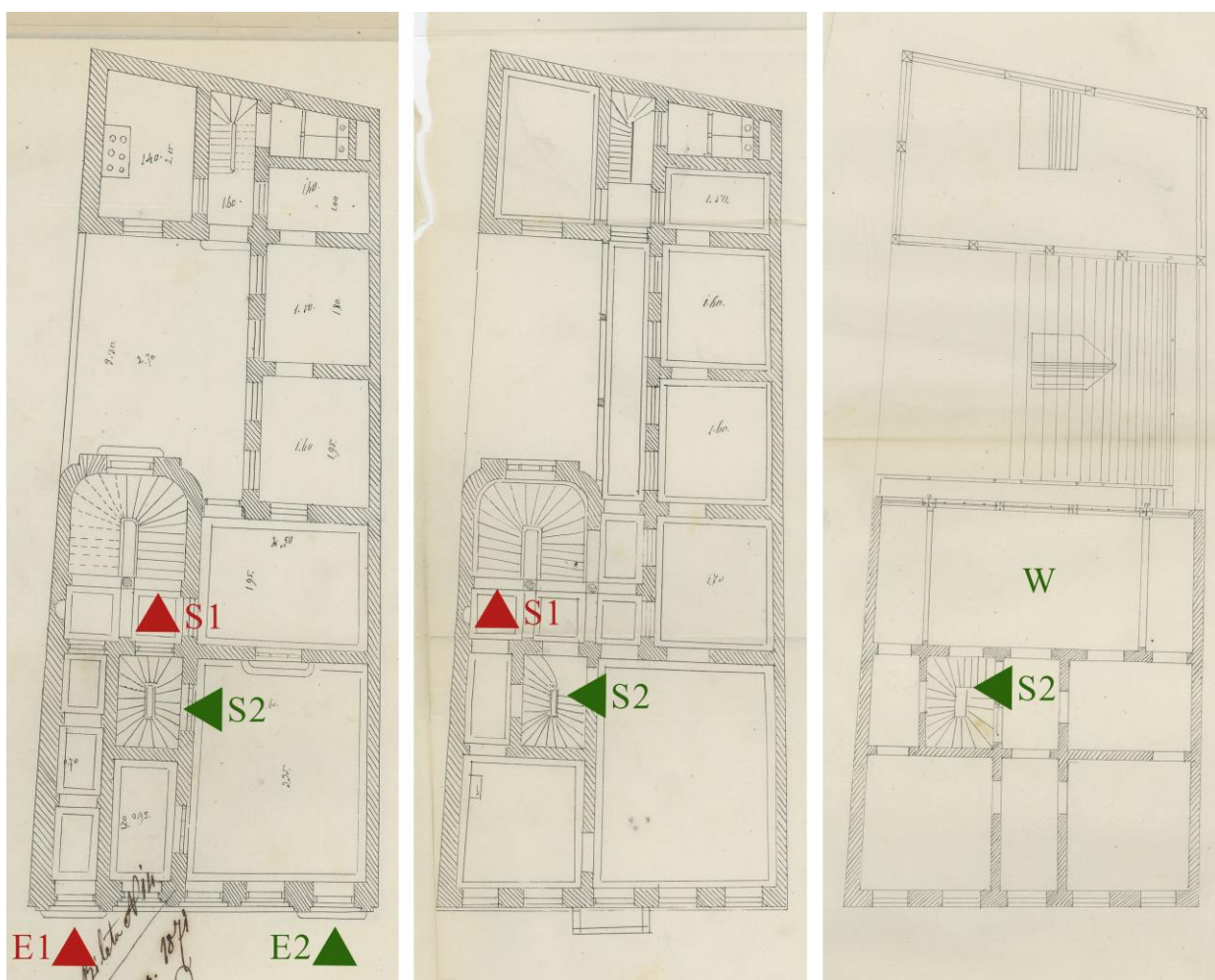
Fig. 9: Architectural project for Franz Duschek’s house in strada Nouă (submitted on 13/25 January 1871): floorplans for the ground floor, first and second floor. SMBAN, fond PMB Serviciul Tehnic, d. 40/1871, ff. 14–15. E1: entrance leading directly to the main staircase; E2: customers’ entrance (as proposed in this paper); S1: main staircase; S2: customers’ staircase; W: main workroom on the upper floor.
