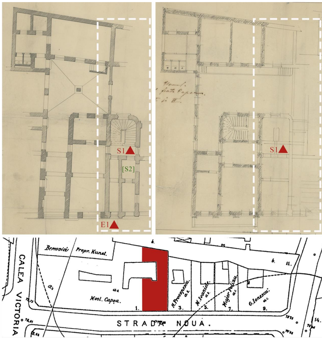
Fig. 10: (top) Architectural project for the extension of the Slătineanu house in str. Nouă (submitted on 14 March 1873): plans for the ground floor and the first floor. The connection to the Duschek house, its partially reproduced floorplan in highlight. SMBAN, fond PMB Serviciul Tehnic, d. 15/1873, ff. 57–58. (bottom) The approximate position of the Duschek house in the post-1873 Capșa ensemble. Planul orașului București (1911), grids XIII C and XIII D, detail.
